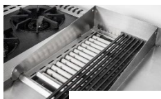
CERAMIC TUBES ARE USED FOR GRILL RANGE
